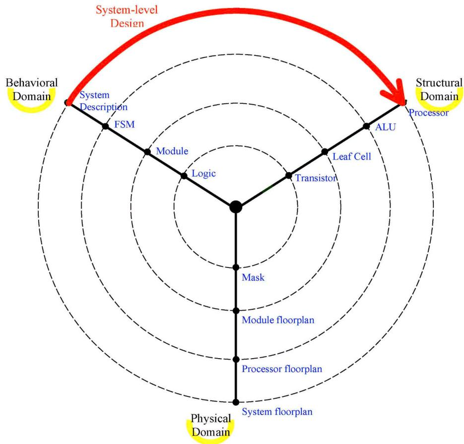
Figure 1: System-level Design in the Y-Chart.
